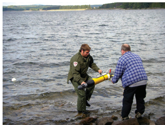
At less than 4 feet long and 40 pounds, the AUV is easily deployed and retrieved from shore.
