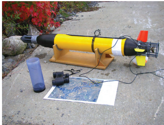
A YSI 6600 water quality sonde is mounted inside an OceanServer AUV for spatial mapping of drinking water reservoirs.
